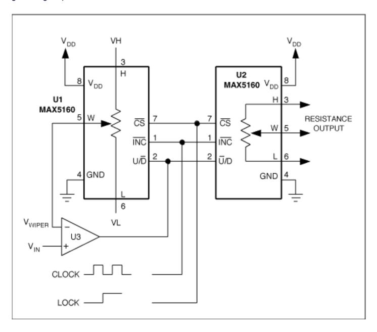
Figure 1. Two indentical digital potentiometers enable this circuit to implement voltage-to-resistance conversion.
